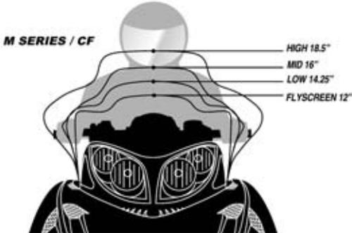
Measurements are taken vertically from dash panel to top of windshield. Style illustrations apply to indicated models only. Use reference point to determine style of windshield to order. Style of windshield for all other models is determined by measuring upward from lowest front center point on windshield to top center point. Accessory windshields do not have pre-drilled mirror mounting holes.
