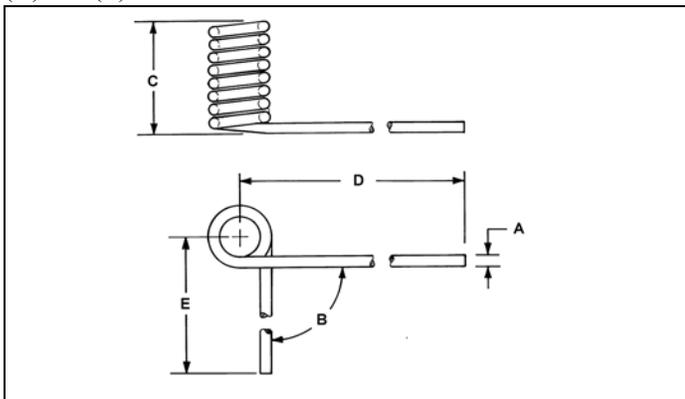
(A) Long spring leg is bent inward (B) Short spring leg is bent inward
